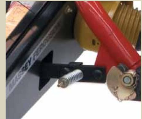
The spring loaded anti-collision break away system allows the mower to pivot backwards if the mower comes in contact with an object protruding from the ground, giving the operator time to stop the tractor before serious damage can occur.
