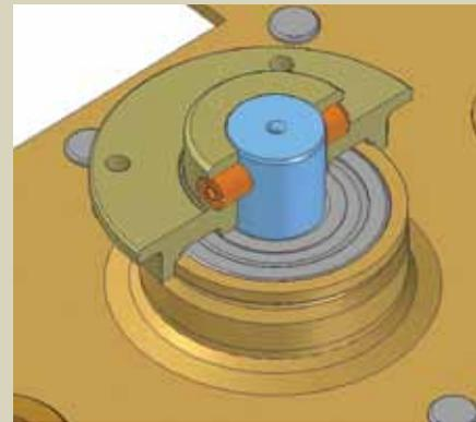
Concerned about rock damage to your cutterbar? No problem. The cutterbar is equipped with a roll/shear pin for every disc that will break outside of the cutterbed, preventing any internal damage and eliminating contamination of the oil bath.
