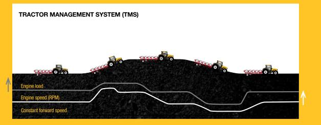
As the load (grey line) varies according to conditions, the TMS will automatically adjust the engine speed (white line) to maintain the forward speed while minimizing fuel consumption and noise levels.
