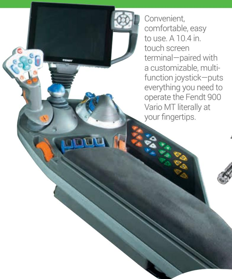
Convenient, comfortable, easy to use. A 10.4 in. touch screen terminal—paired with a customizable, multi-function joystick—puts everything you need to operate the Fendt 900 Vario MT literally at your fingertips.
